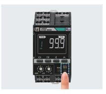
"MANU MEAS" switch on the lower right of the front panel
