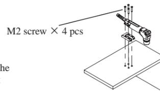
The adjacent installation is possible in this mounting method.
