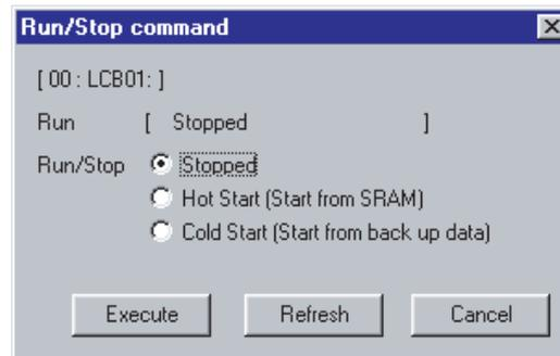
**Note** By a hot start, operation is started continued at the state that was active before the stop occurred. By a cold start, operation is started after all internal operation memory is initialized. (PID is reset to the Manual mode with MV = 0% and a local SP.)
