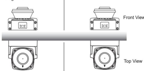
Use of a screen may increase the effect of reflection depending on its material. Select one with matte black finish that is resistant to reflection.
