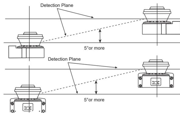
When installing the OS32Cs side by side, it is more effective to set their mounting heights differently. When adjusting the OS32C tilted, it may be more effective to adjust the OS32C downward depending on the condition of the outside light source (natural light or halogen light).
