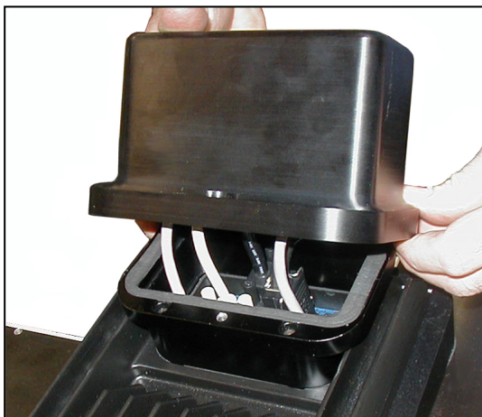
Figure 3-22. Installing Cable Entry Top Cover Assembly
