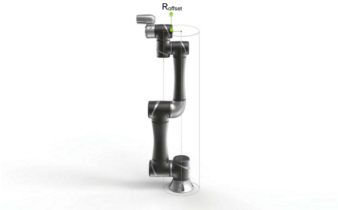
Figure 3: The Definition of R_{offset} .
