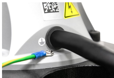
Figure 24: Securing the ground wire with the robot
