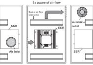
XIf the air inlet or air outlet has a filter, clean the filter regularly to prevent it from cogging to ensure an efficient flow of air.
