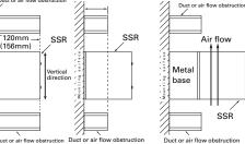
Duct or air flow obstructio Do not surrounded the SSR with the duct in the depth direction, or otherwise the heat radiation of the SSR will be adversely affected.
