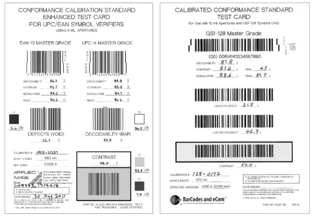
The Calibrated Conformance Standard Test Cards are used to calibrate the light source to a known level of white and black. There cannot be any other item in the field of view when calibration takes place. Failure to comply with these instructions will distort the final verification grade.
