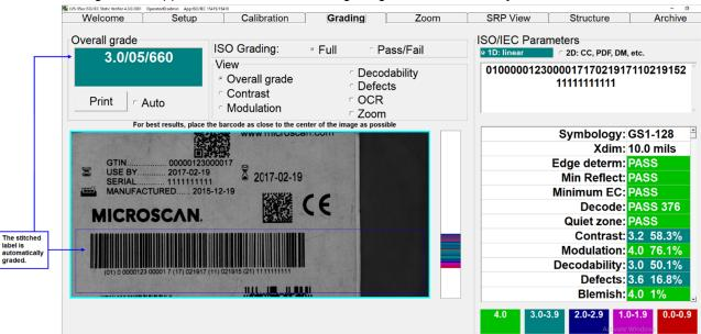
10. When the Stitching feature is complete, the LVS-95XX software automatically turns off the camera; however, the camera must be turned back on. To turn on the camera, click the "Setup" tab and click "On" within the "Camera" section.
