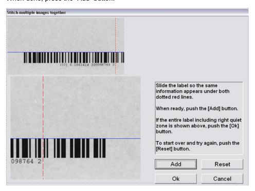
8. In the screenshot below, the right end of the barcode appears along with the appropriate space for a quiet zone, indicating that no additional stitching is required. Press the "Ok" button.
