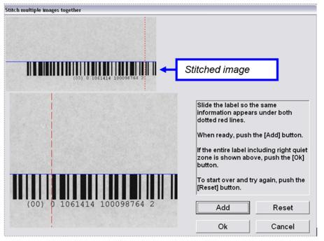
7. In the screenshot below, the label has been moved to its proper stitching position. Notice that the bottom image is aligned to the red line in the same position as indicated in the stitched image. Also notice that the bottom image barcode continues to be aligned perfectly to the blue line. When done, press the "Add" button.
