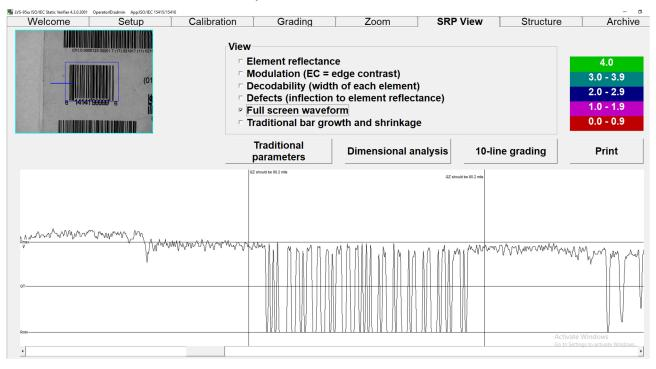
**Note:** If a quiet zone failure occurs, click the viewing box to locate the failure. The SRP window will show the actual quiet zone and required quiet zone.
