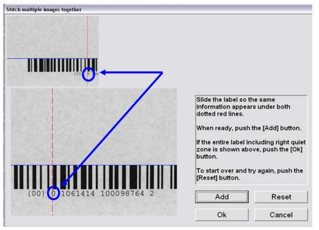
6. The stitched image appears at the top of the screen. The red line shifts over to a new position and you are now prompted to move the label over to its new stitching position.
