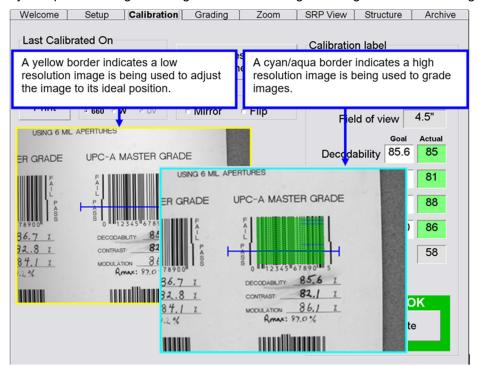
Barcodes can be verified in any orientation, which is an integer multiple of 90 degrees.
