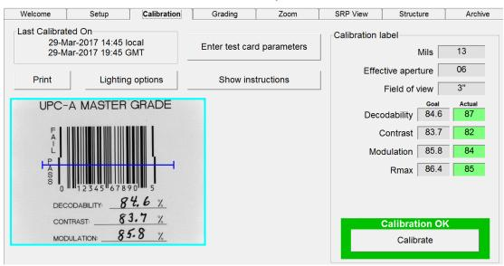
One of the following three Calibrated Conformance Standard Test Cards were supplied with your LVS-95XX system. The test card you receive depends on your field of view.
