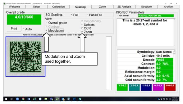
If the Zoom feature, along with either the Modulation, or Defects feature, are checked and a Verification Report is printed, the thumbnail view on the report shows the results in color according to the legend at the bottom of the screen.
