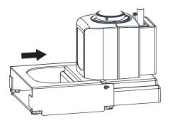
Rotate the mounting brackets to secure the FZ-SLC15 illumination with the provided hexagonal wrench. Securely tighten the screws of the mounting brackets.
