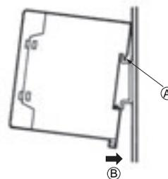
When mounting to a DIN Rail, lower the S82S onto the Rail until the Rail stopper clicks into space, hook section A over the edge of the Rail, and push in the direction of B.
