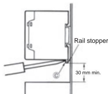
To remove the S82S from the DIN Rail, insert a screwdriver into section C and pull the S82S away from the Rail.
