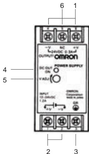
1. **DC Output Terminals:** Connect the load lines to these terminals.
