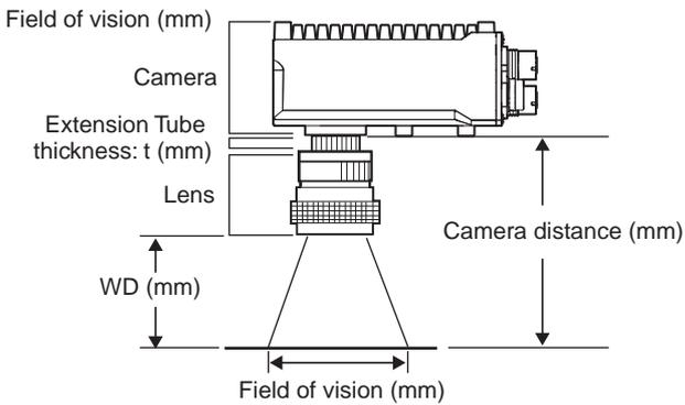
\*1. The lengths of the fields of vision given in the optical charts are the lengths of the Y axis.
