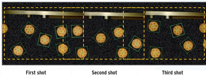
Objects that overlap within more than one field of view are segregated and only inserted in the picking queue once.
