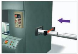
Diameter measurement of metal objects
