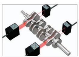
Diameter measurement of crank shaft
