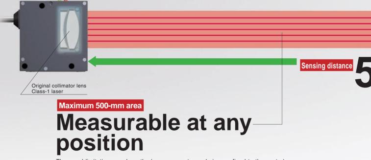
The usual limitations, such as the 'measurement area being confined to the center' or 'large errors due to positioning', that used to plague laser measuring sensors have now been overcome. Measurements can be consistently taken within a 500 mm area, whatever stage the work is at or whichever way it is inserted. It can now be set to positions without interference from the work feed and without limitations of size of work area.
