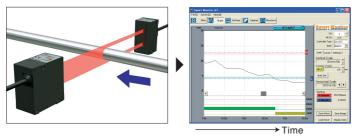
The trend of the measurement data and sudden change can be checked in the timedependent graph, so that the appropriate action can be taken before defective goods
