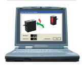
The direction of the sensor head's adjustment is graphically displayed. The adjustment conditions can be confirmed through the shapes of the light reception waveforms.
