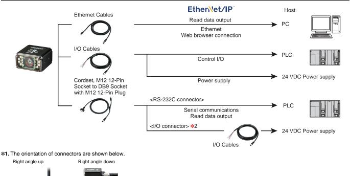
\*2. Connect V430-W8 to I/O connector (M12 12-pin plug) and connect to a power supply.
